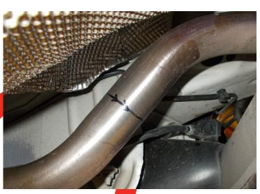
When fitting the rear silencer the original system requires cutting in a specific place. Cut the pipe directly between the two bends as marked in the picture.
